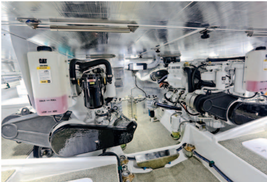
A pair of Caterpillar 450hp engines lives in carpeted splendour and gives a cruising speed of around 20 knots and a top speed of 26 knots
